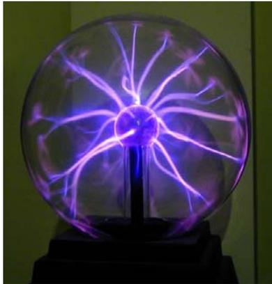
*Figure 5-27: Plasma discharge in an oxygen-filled glass sphere. Image courtesy of Technorama, Switzerland.*
