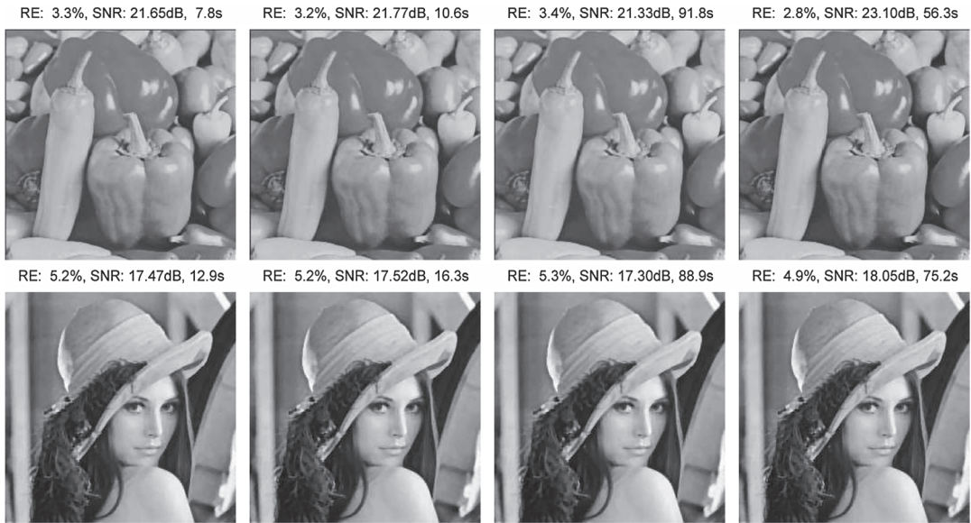
FIG. 5. Restored images by ADMM, HTY, TwIST and FISTA, respectively. The first row: ‘peppers’; the second row: ‘lena’.
